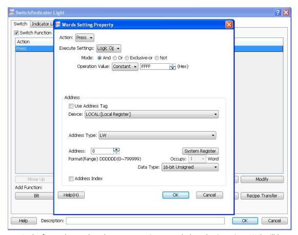
In the figure above, when the component is operated, the value in register LWO will has a logic operation"And" with 0×FFFF. The logic result will be written to register LWO. The operations of otherthree modes are similar to "And" mode but the logic operation.
