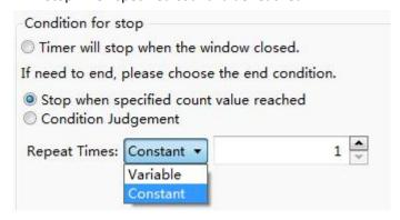
You can use the condition for stopto make the timer end automatically after repeating the specified number of times. Wherein, for the specified number of times, you can directly enter it by Constant, or you can specify a word register to control the timer execution times by Variable.
