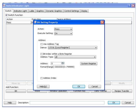
The default action is "Press". The default Execute Setting is "On". The default address is "LBO". They are modified into the required as follows.
