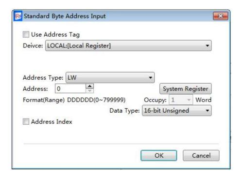
In the Rievtech Studio software, the corresponding byte or word addresssymbolsare given according to the various connected devices. For the Rievtech FL2N series PLC,D represents the data register,SD represents the special address, represents the timer, C\_word represents the 16-bits counter which saves the current value, and C\_dword represents the 32-bits counter which saves the current value. As shown as below.
