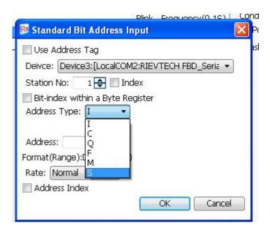
In the Rievtech Studio software, the corresponding bit address symbols are given according to the various connected devices. For the Rievtech PLC FBD\_Serial, I represents the input address, C represents the cursor key address, Q represents the output address, F represents the digital flag address, M represents the block status address, and S represents the shift register bit address. As shown as below.
