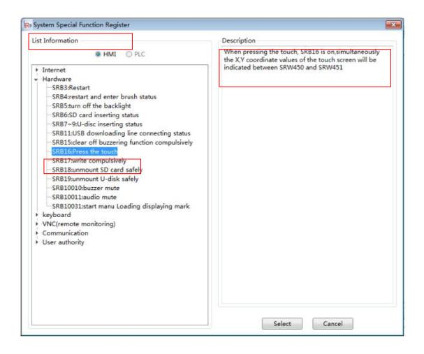
**Note:**"Word Register" and "Bit register" in HMI are two different areas, so the address does not overlap. For example, LW0 and LB0 are two registers that they are not related. SRW0 and SRB0 are also two different special system registers. But each word register can be divided into 16bit registers. For example, LW0 can be divided into 16bit registers: LW0.0  $\sim$  0.15.
