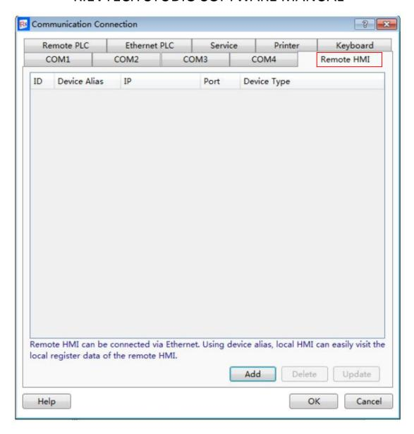
For one of the HMI device, anyone of other HMI devices in the same Ethernet network of the LAN is the Remote HMI. For example, there are two HMI: one named HMI1, another one named HMI2. These two HMI devices are connected in an Ethernet network. For HMI1 device, HMI2 is the "remote HMI" of HMI. For HMI2 device, HMI is the "remote HMI" of HMI2.
