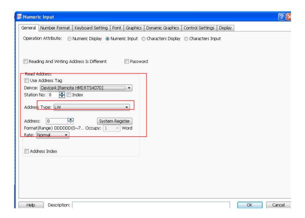
After finishing setting the "Remote HMI", the local HMI can access all the registers of the "Remote HMI", including the LW, RW, SRW, LB, SRB and other registers.
