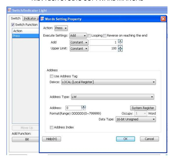
The type of "Execute Settings" includes "Add", "Subtract", "Increase", "Decrease", "Set Up Constants", "Set Up Character Strings", "Set Up Figures By Bit" and "Logic Operation".
