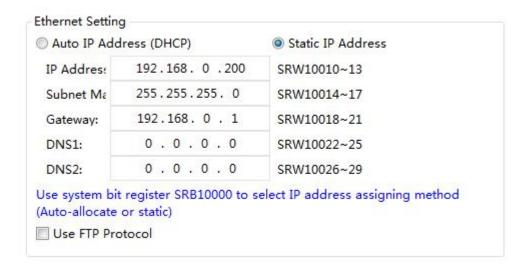
When SRB10000=0, the setting mode is DHCP. When SRB10000=1, the "Static Address" mode is used to assign the IP address. You can switch the IP address setting mode by the SRB10000 register.
