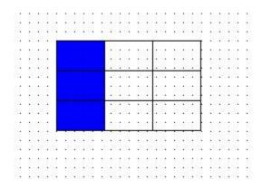
When selecting the mode "Select by Cell", two continuous word registers are occupied. You need to give the first address of the two word registers here. The first word register records the selected rownumber and the second records the selected column number. The first row number and the first column number are 0.
