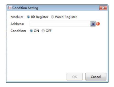
There are two address types: Bit Register and Word Register. The default selection is Bit Register. The logic condition judgment for Bit Register is "ON" or "OFF". The default
