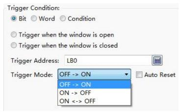
After select the "Bit" option, you can specify a bit register in the "Trigger Address" to control the timer trigger. The "Trigger Mode" can be set "OFF $\rightarrow$ ON", "ON $\rightarrow$ OFF", or "ON $\leftarrow$ OFF". For example, if you set "OFF $\rightarrow$ ON", that means the timer is triggered when the register value changes from 0 to 1.
