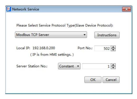
The Service ProtocolType supports Modbus TCP Server. It is referred to:Ethernet Service
