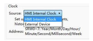
If you select the "HMI Internal Clock" as the HMI clock, SRW0~7 will be used to save the time source of events, historical data, etc.
