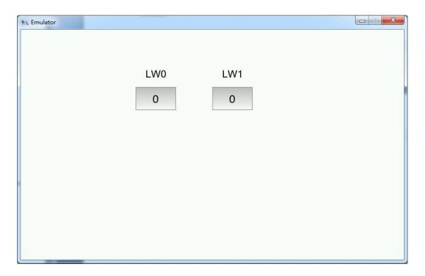
Input the value 100 to LW0. The output value of LW1 will be 300 according to the rules that the output value will be 3 times as much as the input value if the input value is less than or equal to 300.
