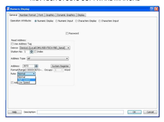
The address setting includes the attributes: "Device", "Address Type", "Address", "Format (Range)", "Address Index", and so on. Please see: <u>Detailed manual/ General functions/ Address editor/ Standard Byte Address Input.</u>
