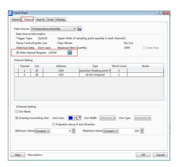
For example, the option "Hide ChannelRegister" is set LW500. Then the curve of Channel 1 is hidden when the bit 0 of the LW500 is ON. The curve of Channel 2 is hidden when the bit1 of the LW500 is ON.
