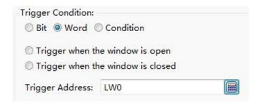
After selecting the "Word" option, you can specify a word register to control the timer trigger. When the value of the specified register is changed, the timer execution will be triggered.
