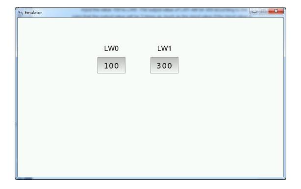
Input the value 400 to LW0. The output value of LW1 will be 800 according to the rules that the output value will be 2 times as much as the input value if the input value is not less than or equal to 300.
