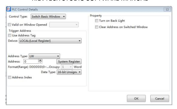
The "Control Type" refers to the action of the "PLC Control". It includes "Switch Basic Window", "Report Current Window No.", "Back Light Control", "Execute Macro Instruction", "Audio Control", "Sheet Print", and "Force Buzzer off".
