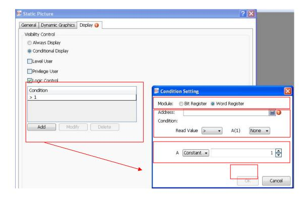
The static picture can be converted into a dynamic one by logic control. Static pictures can be quickly switched by picture stacking and the control address.
