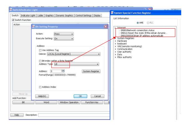
Certainly, the screen is connected with multiple slaves at sometime. The station number is varied. At this moment, you need to use the Index function. This function uses a word address to provide a variable station number. The setting process is shown as follows.
