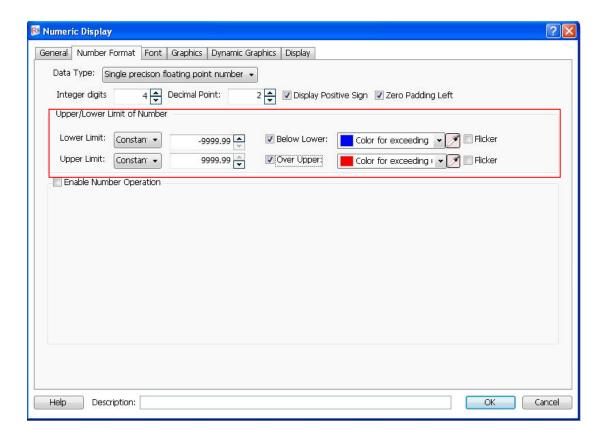
You can set the data upper limit in "Minimum" and the data lower limit in "Maximum". And you can set the font color of the data beyond the limit. When the "Flicker" is checked, the text will flash when the data is less than the lower limit or greater than the upper limit.
