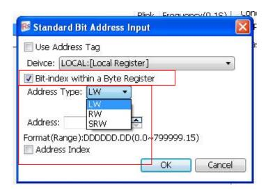
You can use the Address Index function. This function can change the bit address which is connected with the current component according to the value of a word address. For example, the bit address LB0 is connected with the current component. If you check the Address Index and set the address as LW0, as shown as below, the bit address which is connected with the current component will be LB (0 + LW0).
